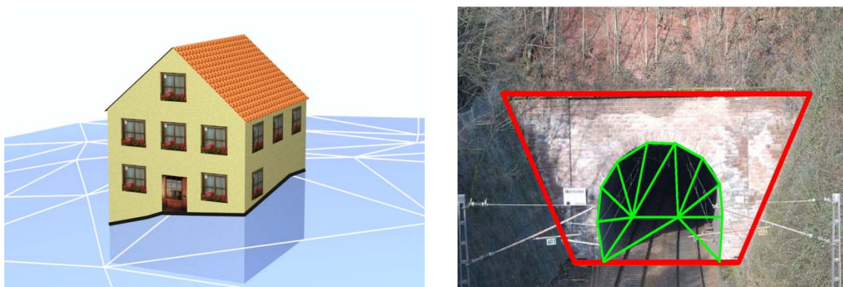
Fig. 4: TerrainIntersectionCurve for a building (left, black) and a tunnel object (right, white). The tunnel's hollow space is sealed by a triangulated ClosureSurface (graphic: IGG Uni Bonn).
