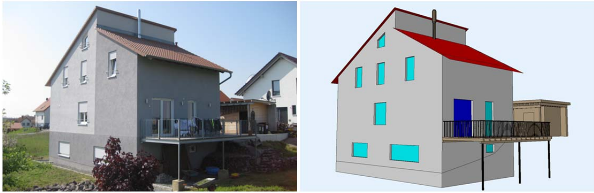
Fig. 35: Example of a building modeled in the Level of Detail 3. The chimney, the balcony and the car port are modeled as building installations (source: Karlsruhe Institute of Technology (KIT), courtesy of Franz-Josef Kaiser).
