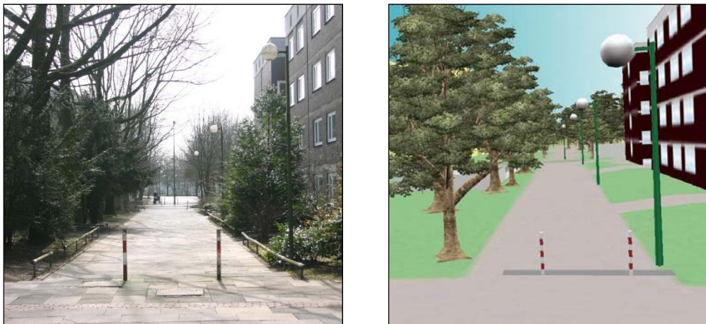
Fig. 67: Real situation showing lanterns and delimitation stakes (left). In the right image they are modelled as CityFurniture objects with ImplicitGeometry representations (source: 3D city model of Barkenberg).
