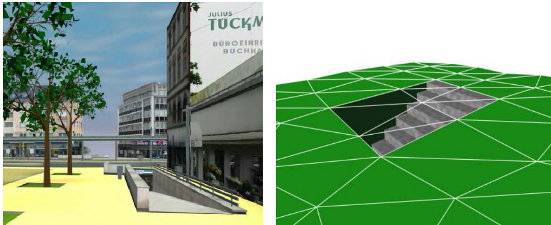
Fig. 3: Closure surfaces to seal open structures. Passages are subsurface objects (left). The entrance is sealed by a virtual ClosureSurface , which is both part of the DTM and the subsurface object (right) (graphic: IGG Uni Bonn).
