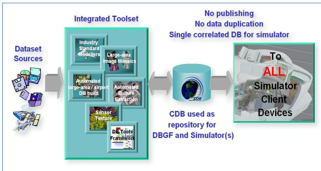
Figure 1: CDB Approach to Synthetic Environment Generation
