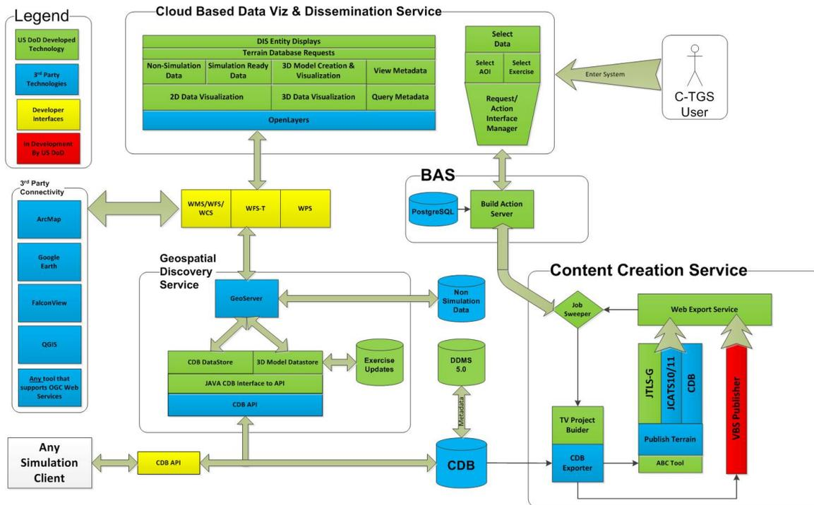
**Figure: DoD C-TGS Architecture (Chambers and Sherman, 2014)**
