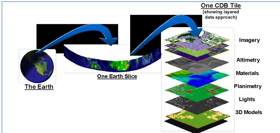
Figure 6: CDB Standard Tile/Layer Structure
