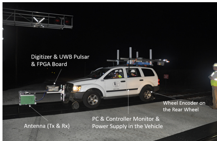
UVM GPR system mounted on the railroad vehicle
