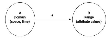
Figure 4 — Conceptual model of a coverage
