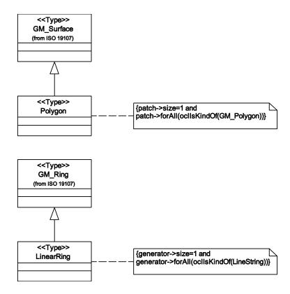
Figure 55 — A GM\_Surface with a single GM\_Polygon patch
