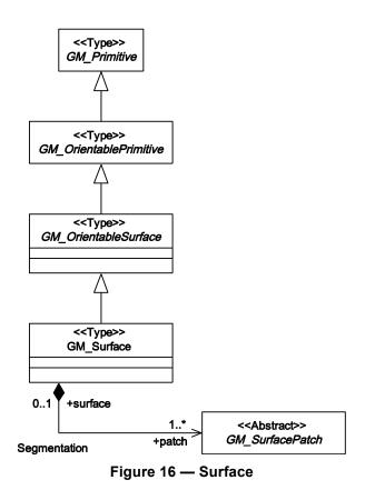
As discussed above, "GM\_Surface" is represented by a "Surface" object element in GML. The "patch" role is represented as an array property "patches" in GML.
