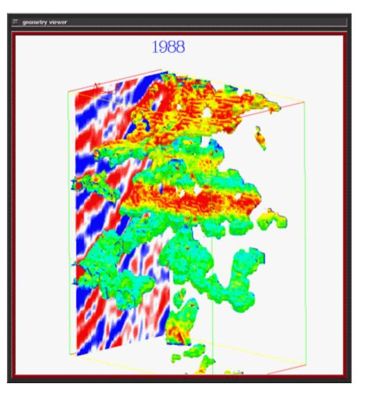
Oil and Gas stacked reservoirs isolated by region growing in a 1988 seismic survey and 1994 survey. Changes in oil, gas, and, water content as well as shrinkage of the stacked reservoir are easily identified.
