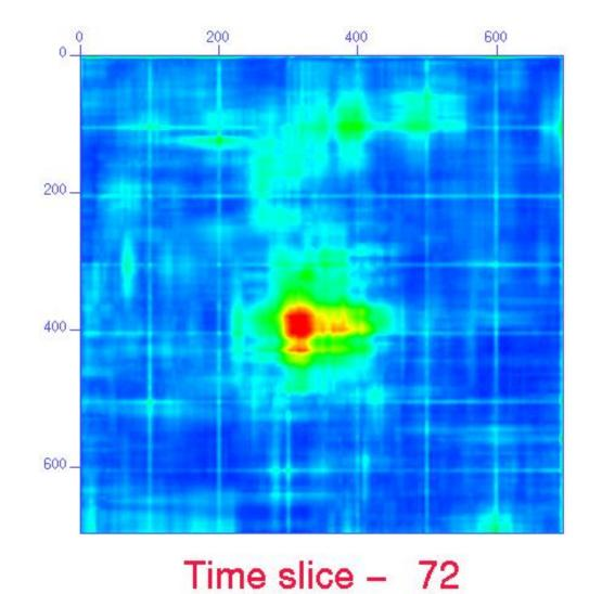
By tracking the DNAPL through the cube of data (actually here only 1.5 meter of the 2.5 meter is shown) we can determine what the path was that the DNAPL took through the sand. This path is considered to be a hydrologic conductive zone, and by inference, must have some different properties from adjacent zones which were not invaded by the DNAPL. The Movie is a series of time slices (or depth slices) through this hydrologic model. The index corresponds with the depth (from top sand)
