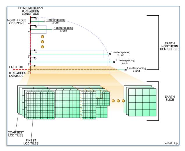
Figure 2-4: Earth Slice Example (Five Levels of Detail)
