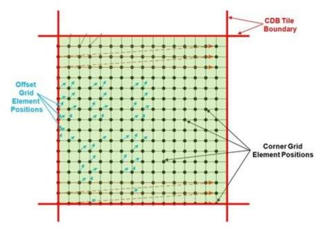
Figure 5-11: Grid Element Coverage within a CDB Tile
