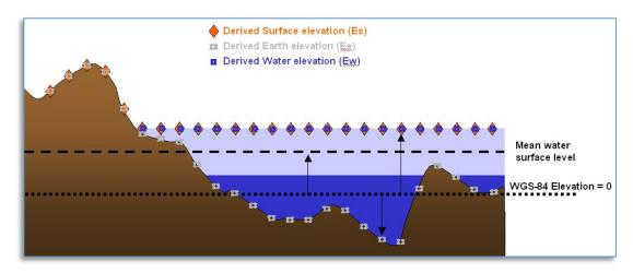
Figure 5-24: Derived Earth Elevation, Water Elevation and Surface Elevation Values
