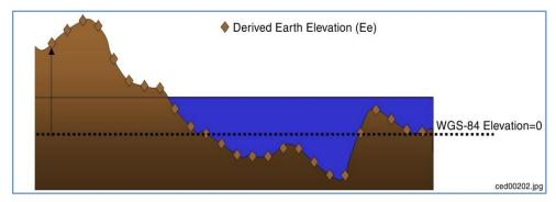
Figure 5-21: Derived Earth Elevation Values
