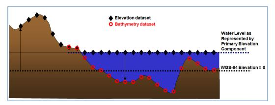
Figure 5-20: Primary Terrain Elevation and Subordinate Bathymetry Components
