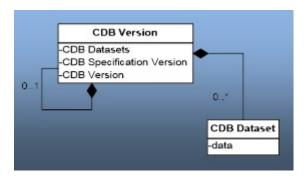
Figure 3-1: UML Diagram of CDB Version Concept
