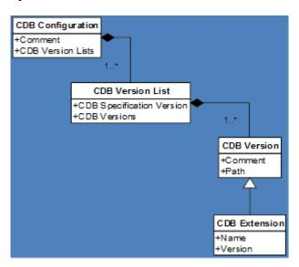
Figure 3-7: UML Diagram of CDB Configuration Concept
