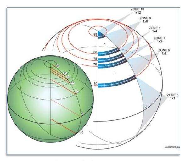
Figure 3-8: Allocation of CDB Geocells with Increasing Latitude
