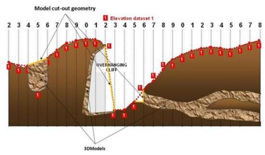
Figure 5-9: Modeling of Wells, Overhanging Cliffs and Tunnels
