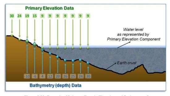
Figure 5-22: Example of Primary Terrain Elevation and Bathymetry Components
