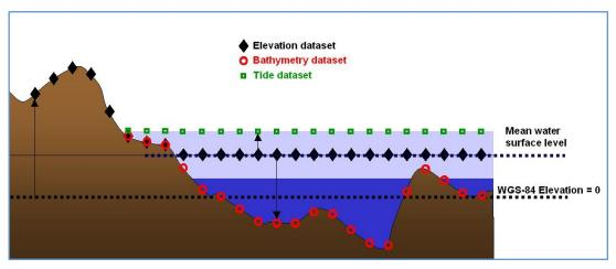
Figure 5-23: Terrain Elevation, Bathymetry and Tide Components
