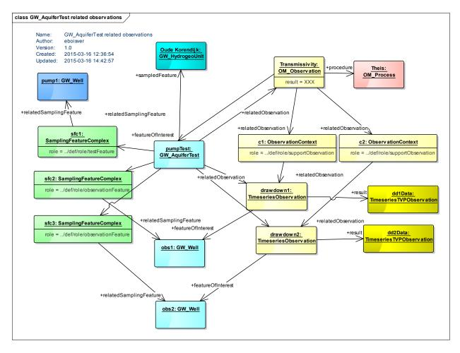
Figure 26: Typical pump test instance: 1 sampling feature and 2 observation features.
