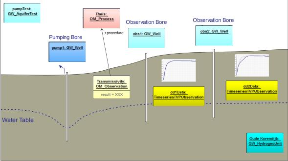
Figure 22: Typical setup of a pumping test.
