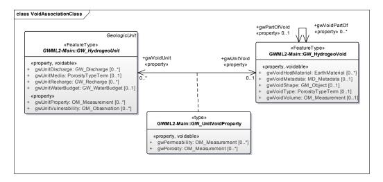
Figure 18: Association class between a GW\_HydrogeoUnit and GW\_HydrogeoVoid.
