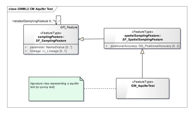
Figure 23: GW\_AquiferTest model.
