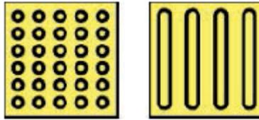
**Figure 1 — Braille Blocks: Stop (left) and Walk (right)**
