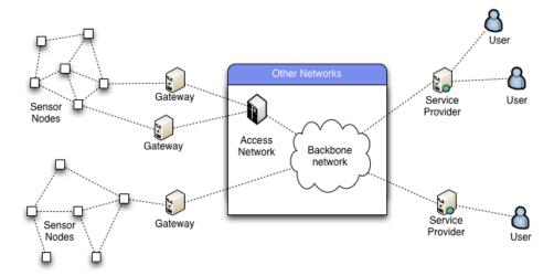
Figure 1, Sensor Network Connectivity
