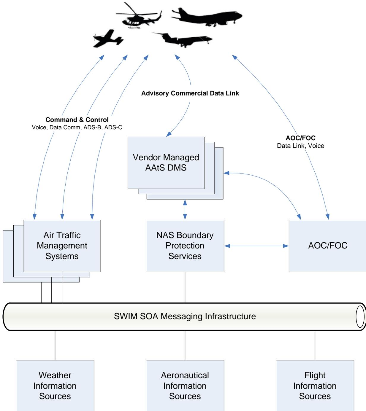
Figure 1 is a “to-be” representation of air-ground information exchange in the far-term NextGen environment including the important role AAtS will fill. On the left side of the figure, primary command and control methods are depicted (e.g., voice). The middle of the figure portrays the bi-directional commercial data link via AAtS used solely for advisory information. The Airline Operations Center (AOC)/Flight Operations Center (FOC), pictured here, may receive advisory
