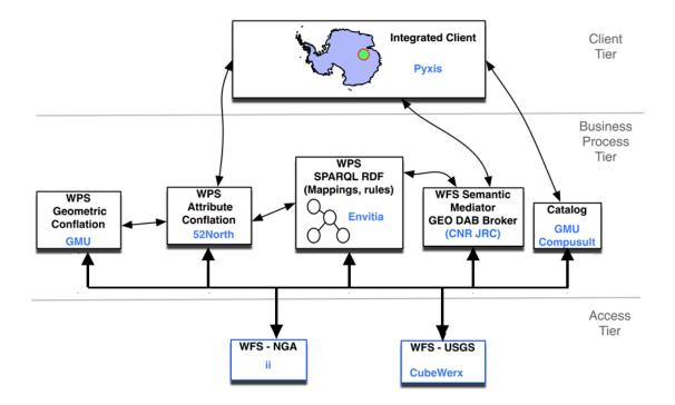
Figure 5. OWS-9 CCI conflation and broker architecture
