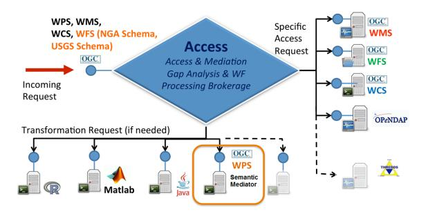
Figure 12. Simplified diagram of the GEO Access Broker with OWS-9 enhancements
