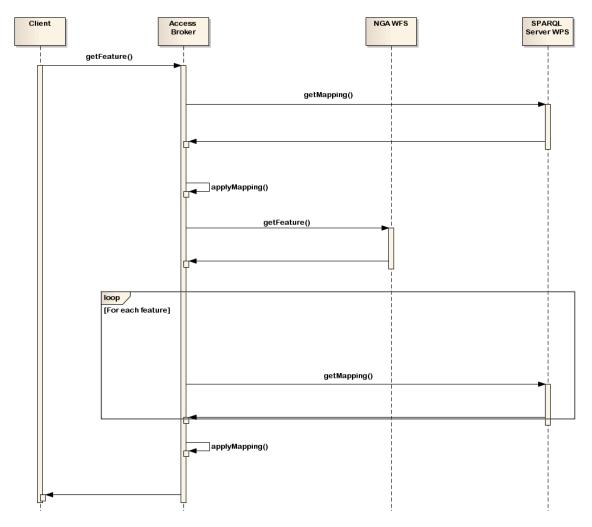
Figure 16. Sequence Diagram for the GEO Access Broker
