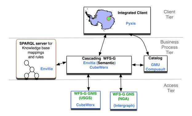
Figure 2. OWS-9 CCI Geonames semantic mediation architecture
