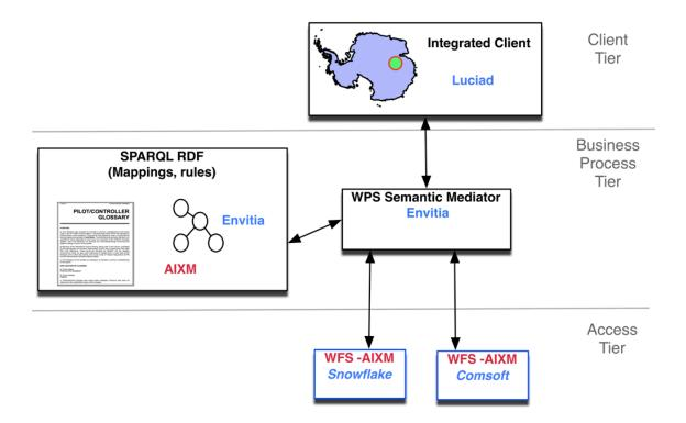
Figure 4. OWS-9 CCI Aviation semantic mediation architecture
