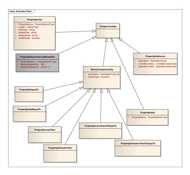
Figure 7. UML class model of proposed extension to Filter comparison operations
