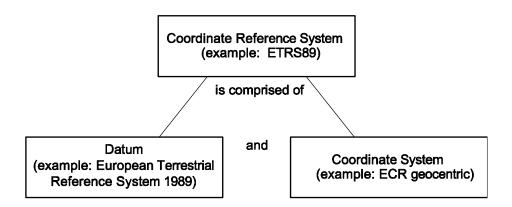
Figure 2 — Conceptual model of a coordinate reference system
