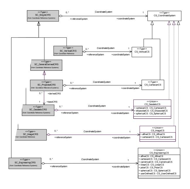
Figure 8 — Coordinate System type associations with Coordinate Reference System type
