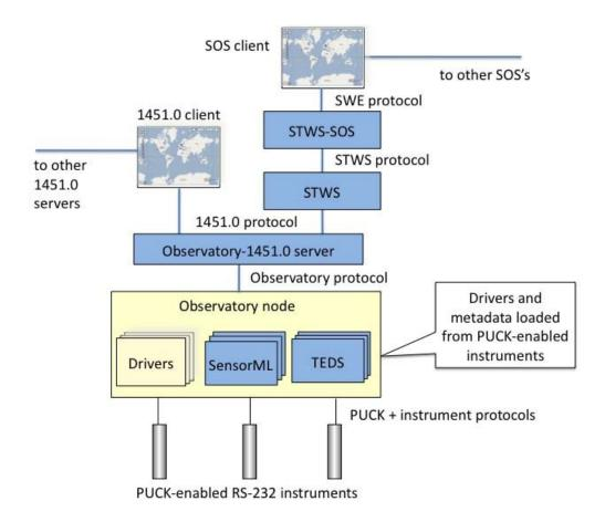
Figure PUCK-1: Basic architecture of PUCK-1451-SWE test-bed
