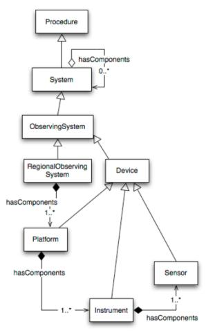
Figure [Complex Systems-1]. Simple UML for systems components. The top classes depict the SensorML conceptual model where a system is a procedure. And a system has components.
