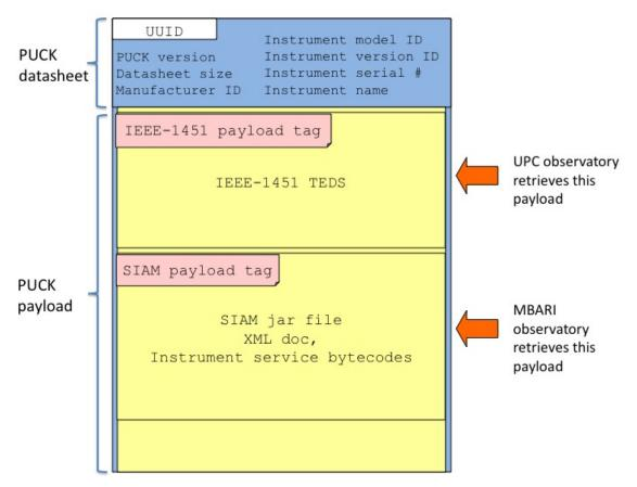
Figure PUCK-4: PUCK memory map example showing multiple "tagged" payload components
