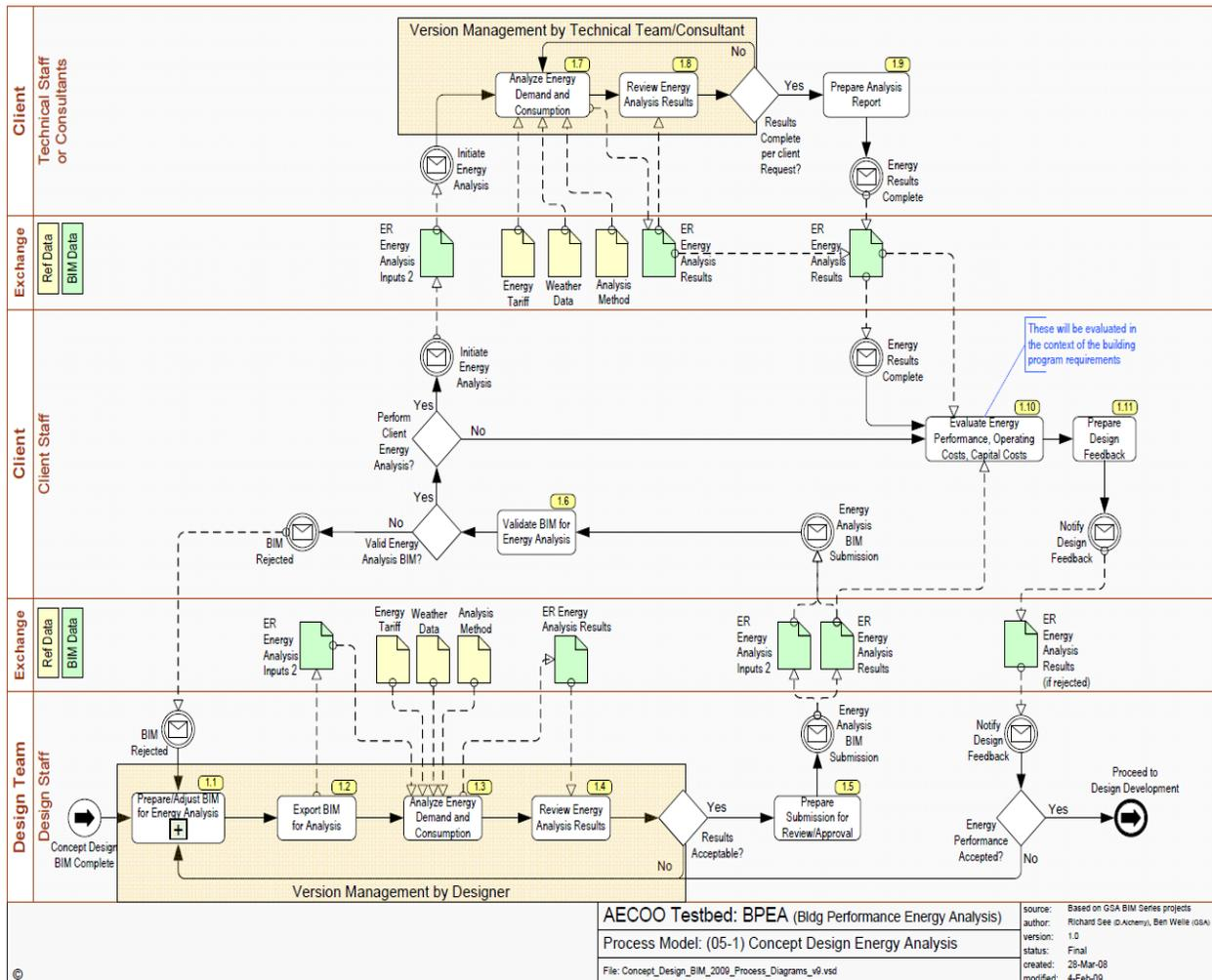
Figure 4 - Concept Design Phase Energy Analysis
