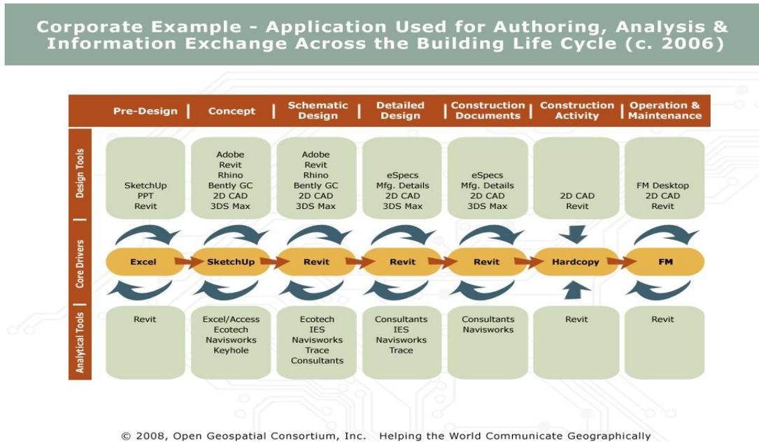
**Figure 8 – The Corporate Example for Authoring, Analysis and Information Exchange Across the Building Life Cycle**
