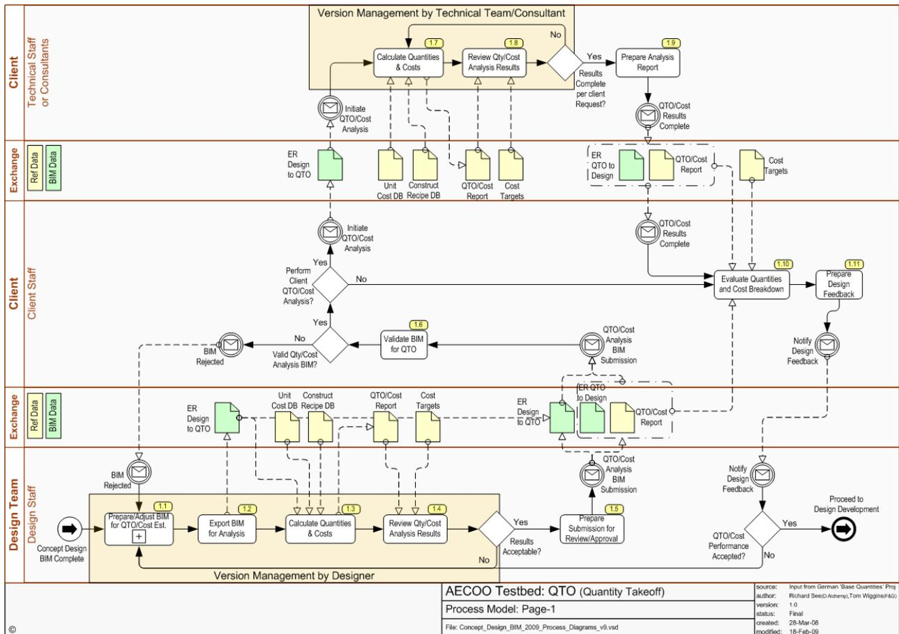
Figure 5 – Concept Design Phase Quantity Take-Off
