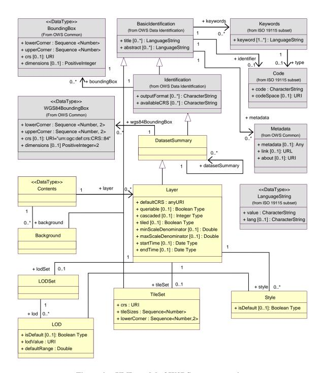
Figure 4 —UML model of W3DS contents section
