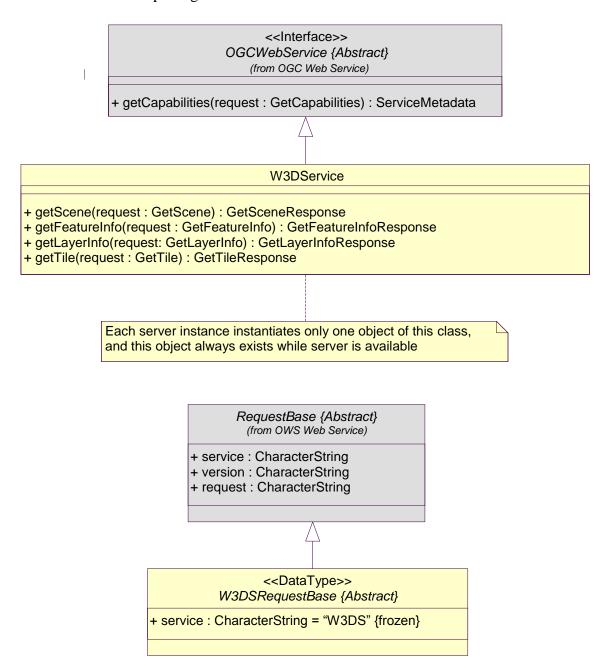
Figure C.3 — W3DS Service package class diagram
