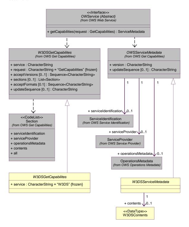
Figure C.4 — W3DS Get Capabilities package class diagram
