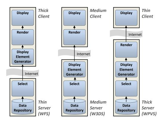
Figure 2 — Different balancing schemes between client and server
