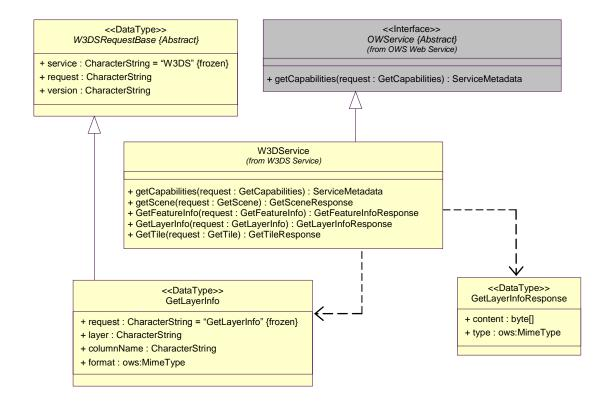
Figure 9 — GetLayerInfo operation request UML class diagram
