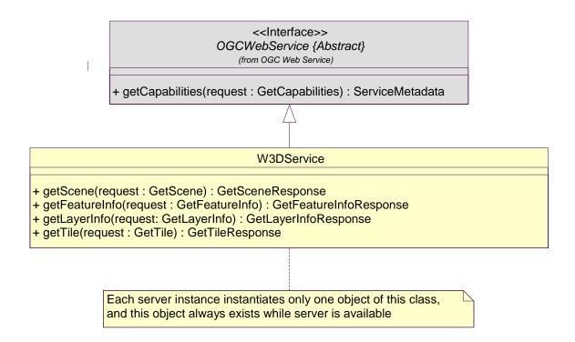
Figure 3 — W3DS interface UML diagram
