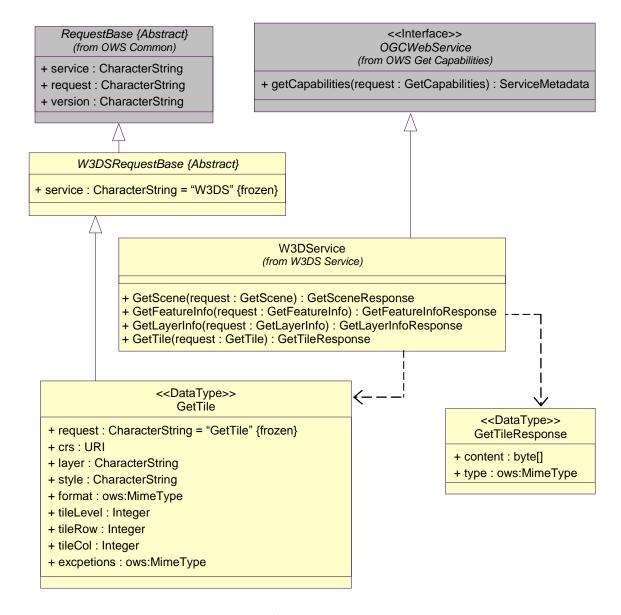
Figure C.9 — W3DS Get Tile package class diagram
