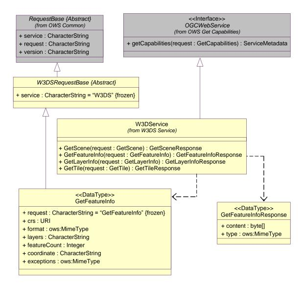
Figure C.7 — W3DS Get FeatureInfo package class diagram
