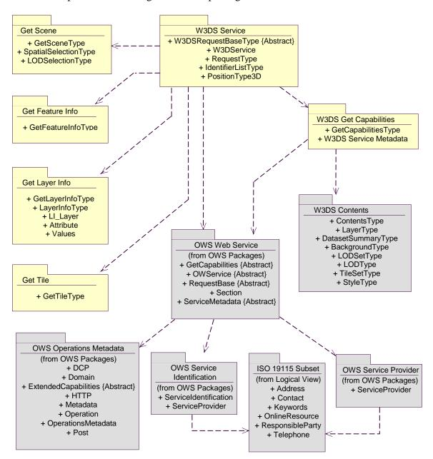
Figure C.2 — W3DS interface package diagram
