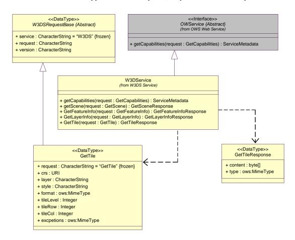
Figure 10 — GetTile operation request UML class diagram
