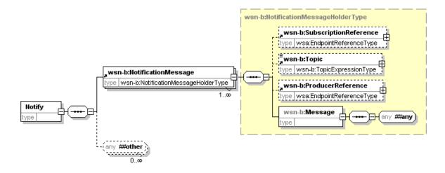
Figure 71 - Notify request element as defined by WS-BaseNotification in XMLSpy notation
