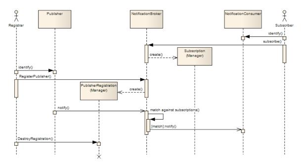
Figure 77 - Interactions in brokered Pub/Sub using WS-Notification
