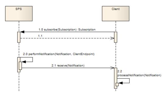
Figure 26 - Exemplary sequence of interactions between an SPS and a Client
