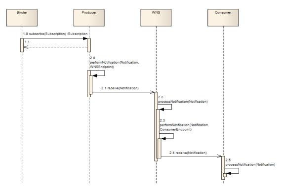
Figure 29 - Exemplary sequence of interactions between a WNS, client, binder and producer
