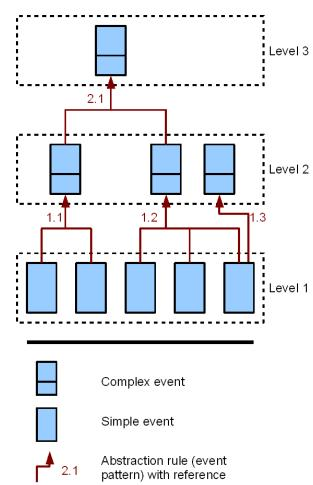
Figure 47 shows a causality model with simple events (level 1), complex events (level 2 and 3) as well as the abstraction rules with reference numbers.
