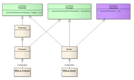
Figure 37 - Mapping the Producer and Broker role to WMSs
