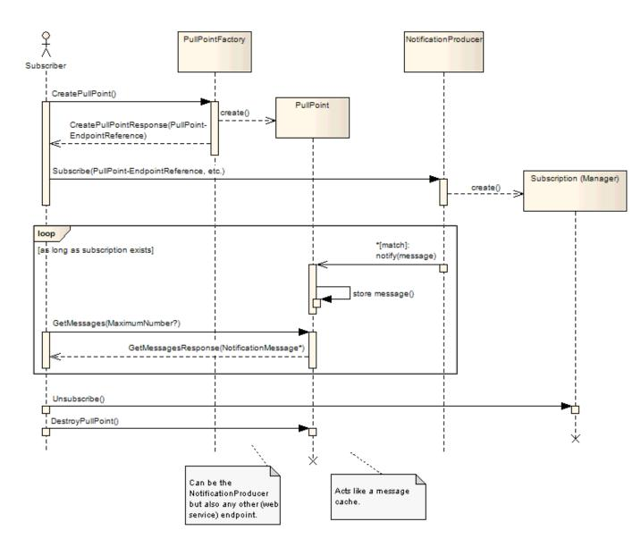
Figure 75 – Pull style notification with WS-Notification using the PullPoint mechanism
