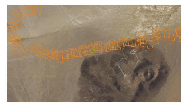
Figure 12. Footprints calculated using a SensorML-encoded CSM Frame Sensor Model, based on retrieving the platform's navigation data (i.e. location and attitude) from an SOS. Rather than treating such data as metadata for the imagery, treating sensor model parameters and other measurements as observations in their own right, enables increased capabilities for discovery and alerts.
