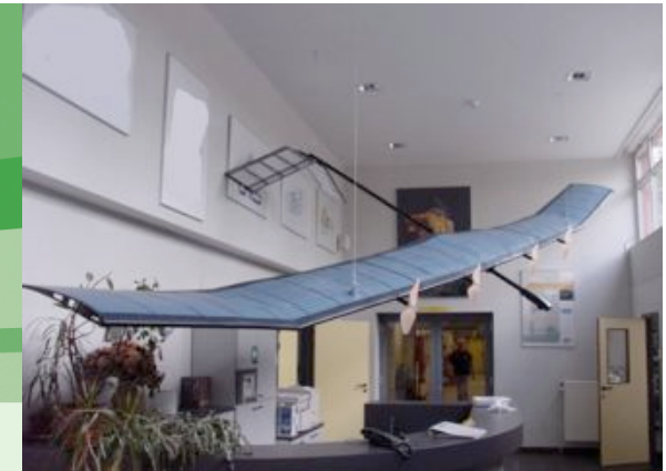
Mercator-1 prototype : ~16 m wingspan, ~2 kg payload (VITO)
