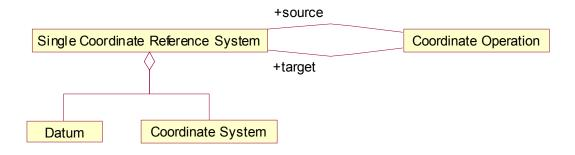
Figure 2 — High-level model for spatial referencing by coordinates
