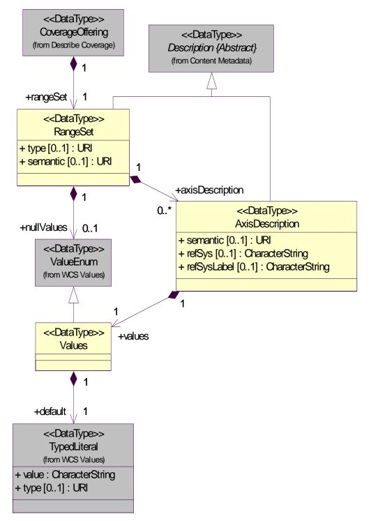
Figure D.6 — Range Set package class diagram
