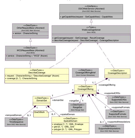
Figure D.5 — Describe Coverage package class diagram
