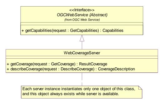
Figure D.1 — WCS interface UML diagram
