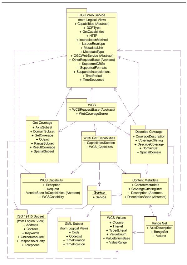
Figure D.2 — WCS interface package diagram
