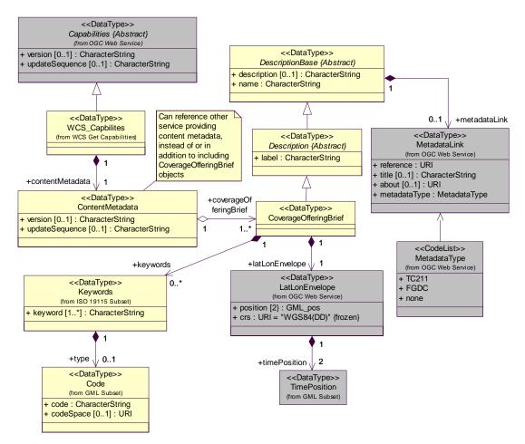
Figure D.11 — Content Metadata package class diagram
