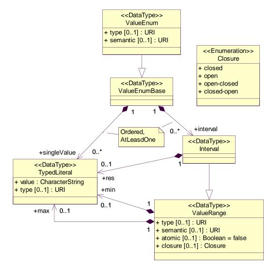
Figure D.7 — WCS Values package class diagram
