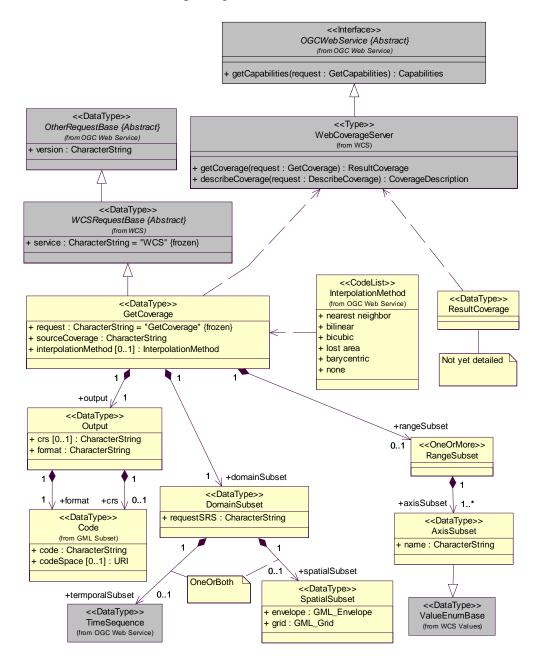
Figure D.4 —Get Coverage package class diagram
