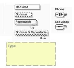
Figure 2. XML Schema graphic symbols
