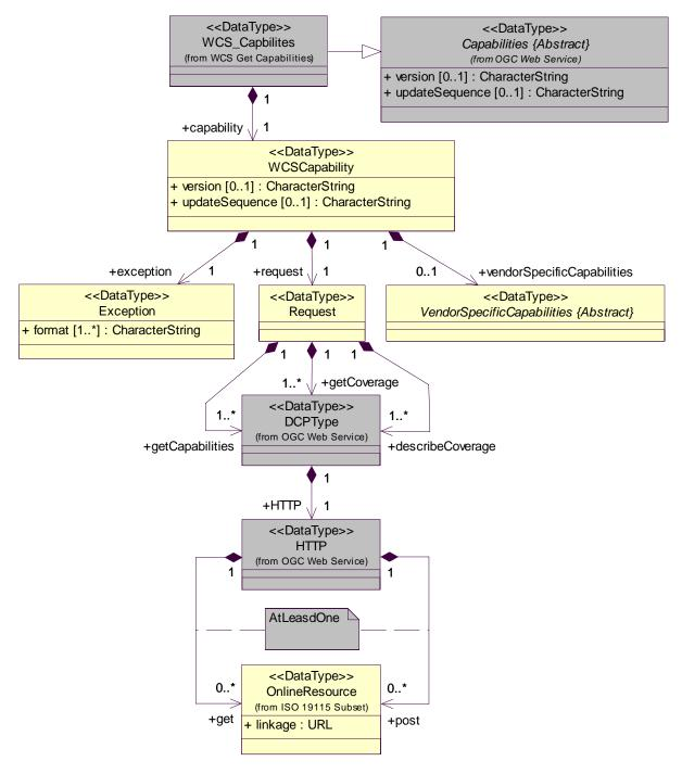
Figure D.10 — WCS Capability package class diagram
