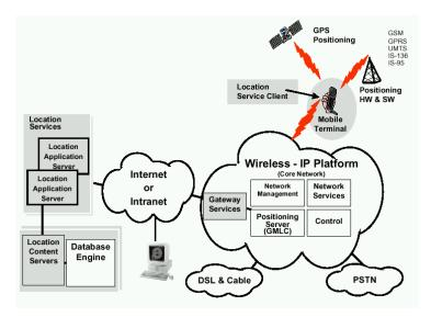
Figure 26 - OpenLS system concept
