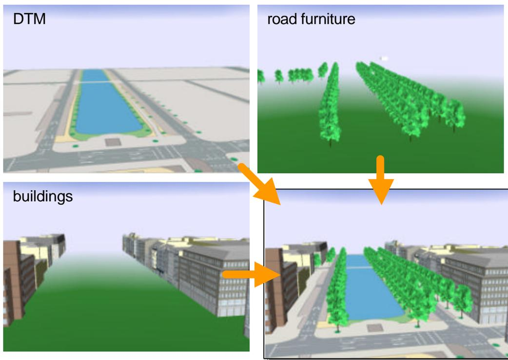
**Figure 1 — Different types of geodata are merged in one 3D scene graph**
