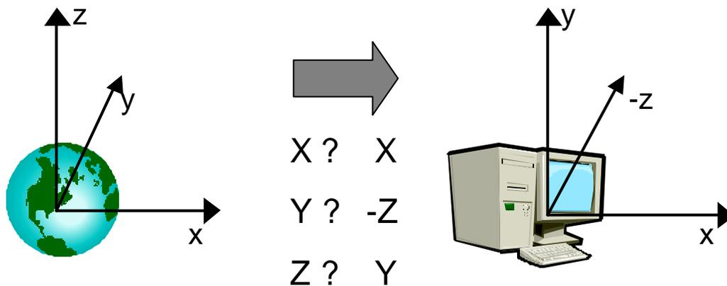
**Figure 5 — Axes transformation from real world coordinates (left) to 3D computer graphics coordinate system (right)**
