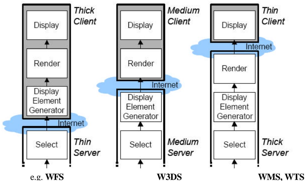
**Figure 3 — Different balancing schemes between client and server**
