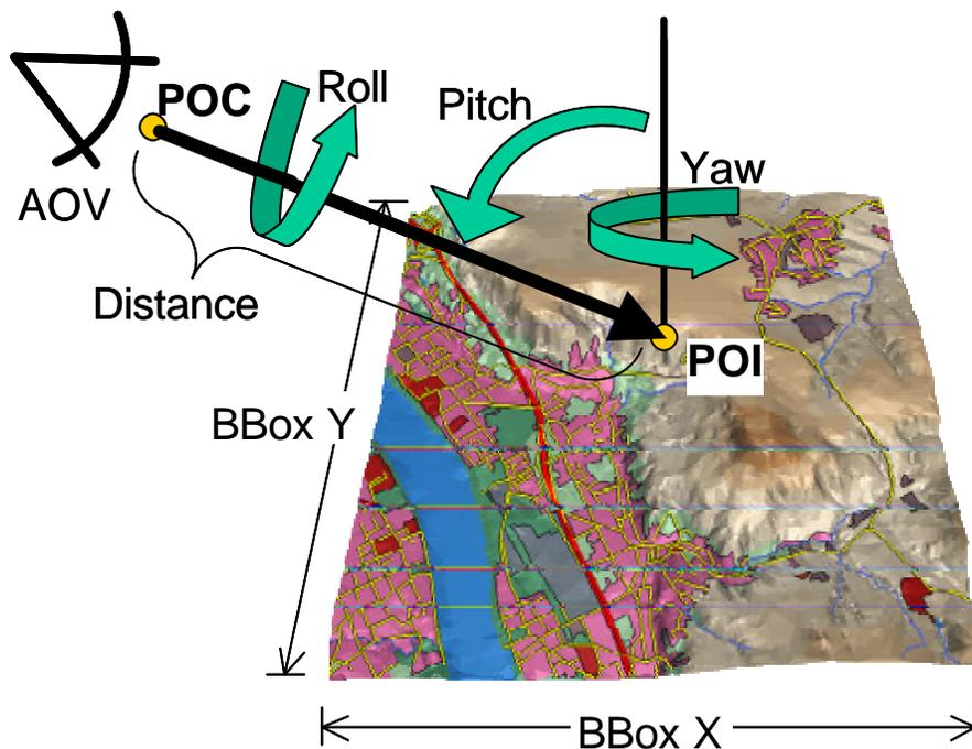
**Figure 4 — The different viewing parameters of the GetScene request**
