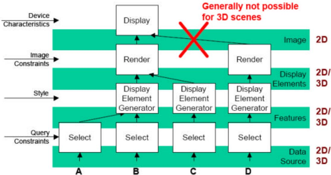
**Figure 2 — The component structure of the portrayal pipeline allows the integration of data on different levels in order to obtain an integrated visualization (Doyle & Cuthbert 1998 [1]). Besides on the image level objects can have both two or three dimensional geometries**
