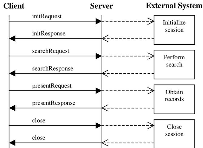
**Figure 27 - WWW Profile Sequence Diagram**
