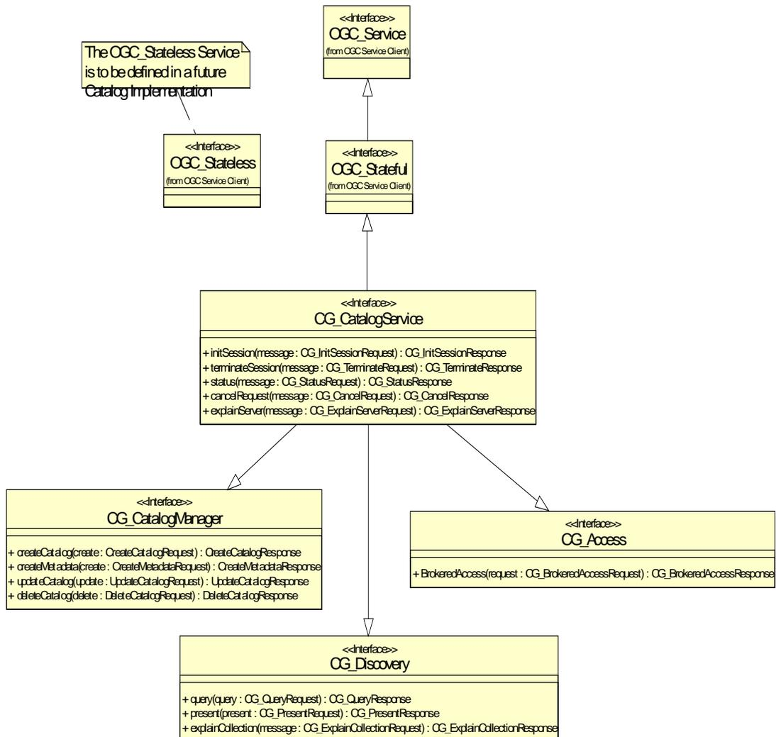
Figure 7 -Main Static Class Diagram of the Coarse-Grained General Interface Model
