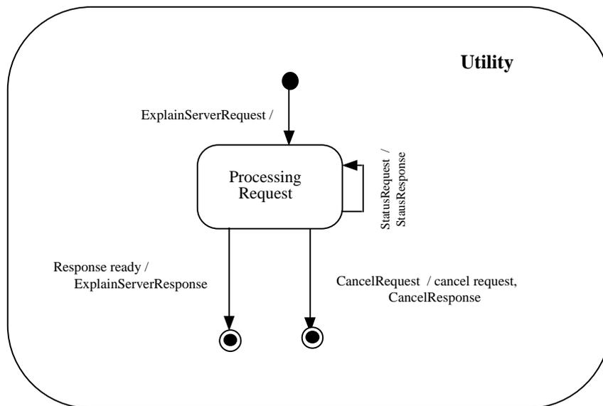
Figure 22 - Utility State Diagram
