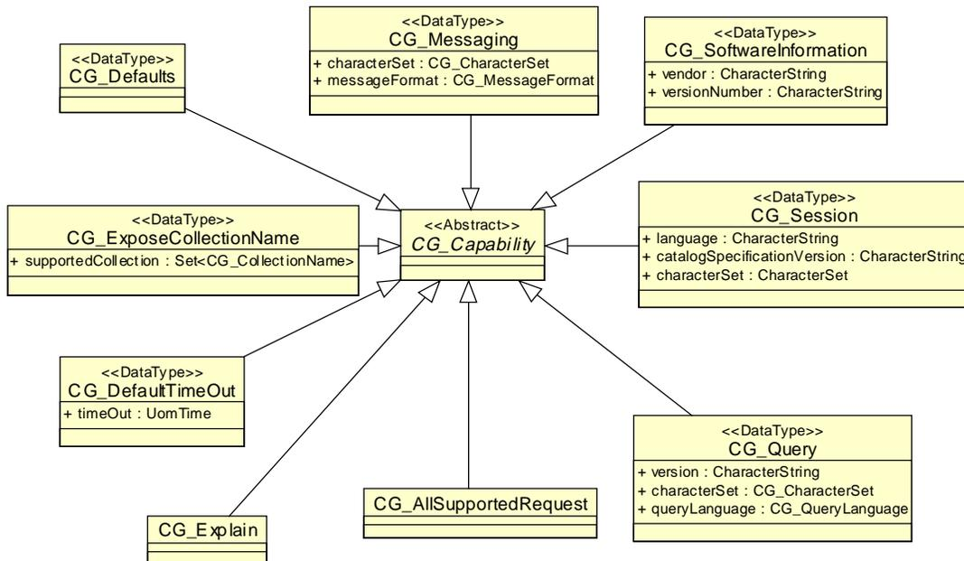
Figure 11 - Static Class Diagram showing CG\_Capability Class and Its Instantiated Subtypes.
