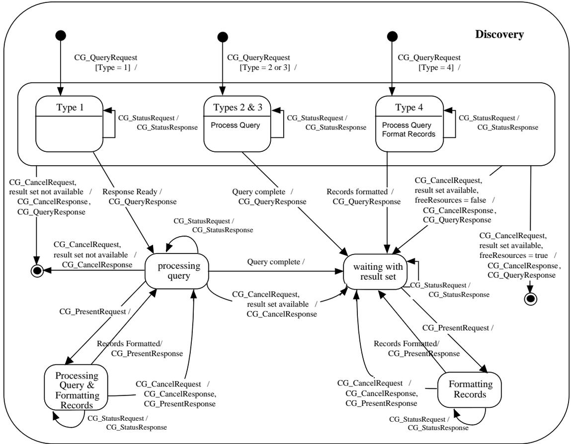
Figure 17 - Discovery State Diagram (Complete)
