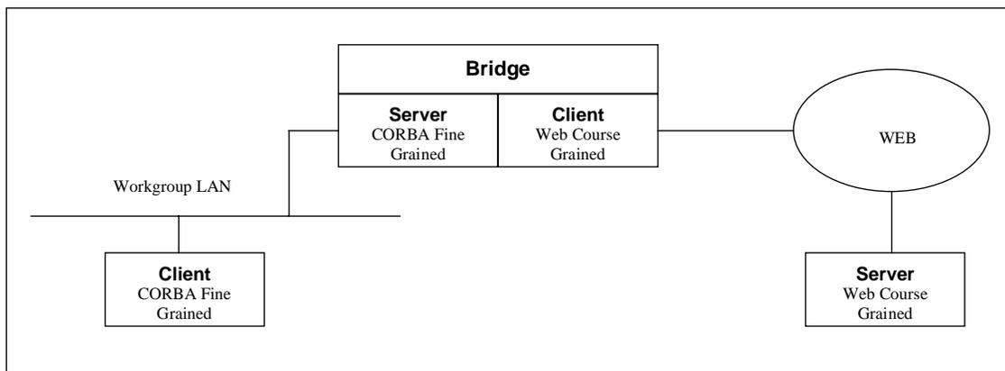
**Figure 4- An Example of a One-Way Bridge**
