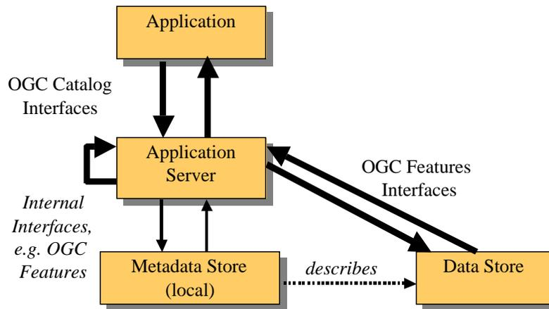
**Figure 2 - Reference Model Architecture**
