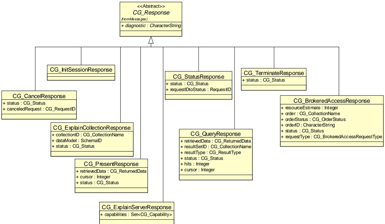
**Figure 10 -Response Message Classes and Their Attributes (Parameters) Defined for OGC Coarse-Grained Catalog Interface Model.**
