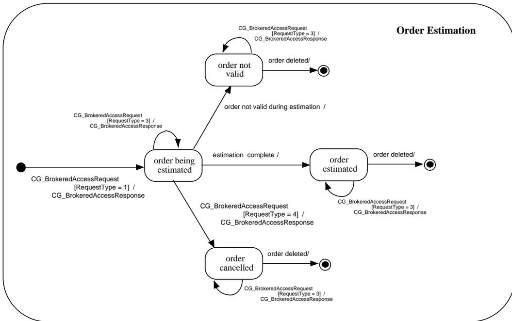
**Figure 19- Order Estimation State Diagram**
