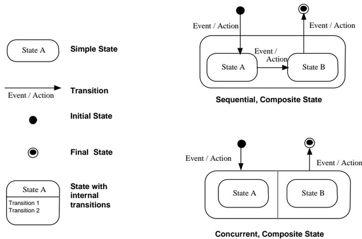
Figure 14 - UML State Diagram Notation
