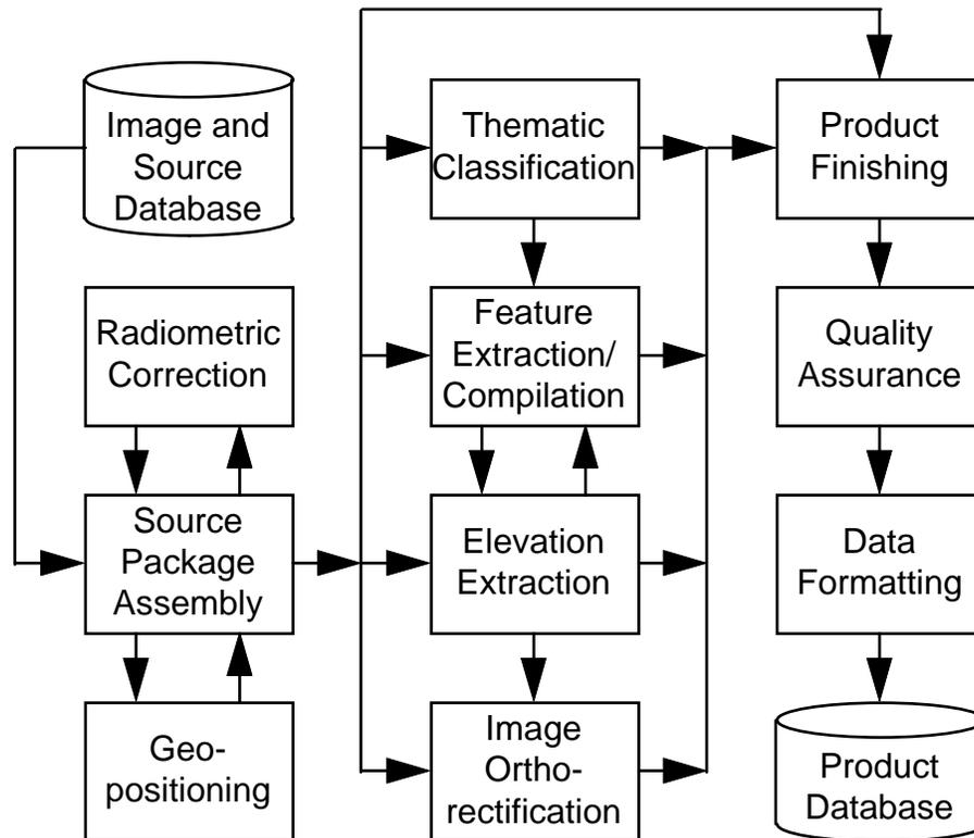
**Figure 7-1. Image Exploitation Block Diagram**
