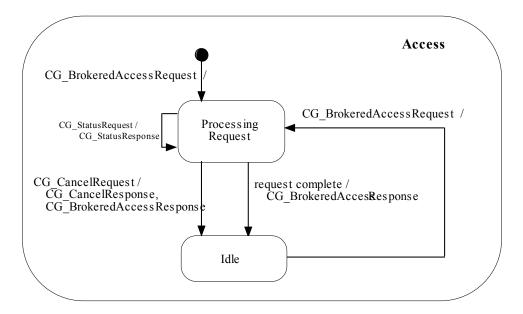
Figure 21 — Access state diagram
