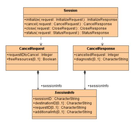
Figure 13 — "cancel" operation UML static model
