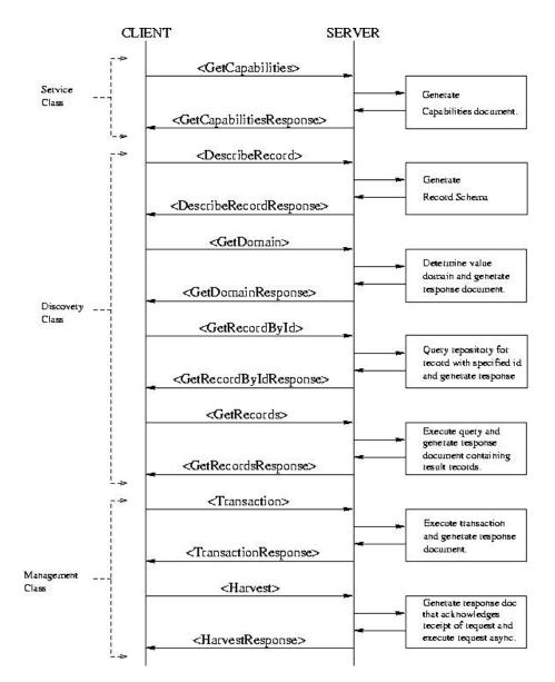
Figure 29 — Protocol sequence diagram
