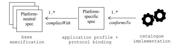
Figure 33 — Relationships between base specs, profiles, and implementations
