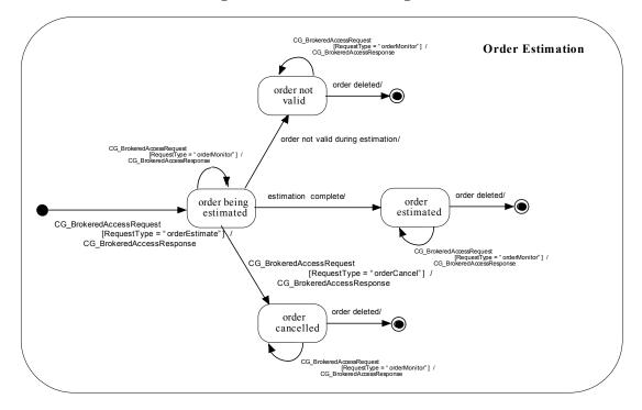
Figure 22 — Order estimation state diagram
