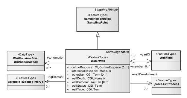
Figure 3: GWML water well model fragment
