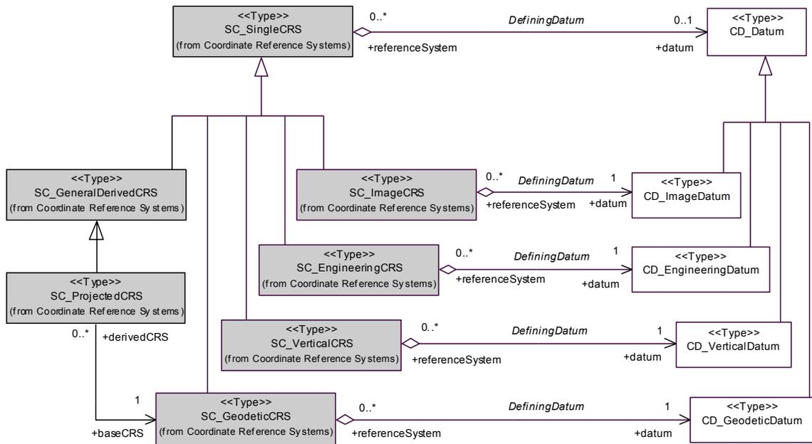
Figure 10 — Datum type associations with Coordinate Reference System type
