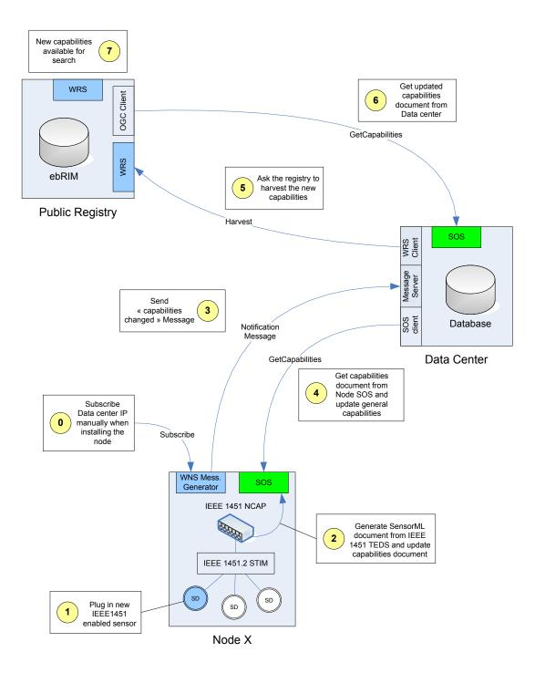
The next diagram illustrates how individual nodes can insert there observations in the main database using the data center SOS-T interface. This way of operation is very useful when nodes cannot keep a permanent network connection with the data center (e.g. GSM).
