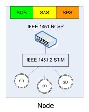
Each node provides connectivity with other network components through optional SWE interfaces. Implementations of these interfaces are expected to be very light weight since the available processing power and storage capacity on each node is very low.
