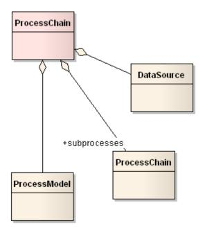
Figure 7-1. ProcessChain aggregates process models, other process chains, or data sources
