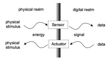
Figure 5-2: Sensor and actuator model (derived from (Ricker/Havens, 2005))
