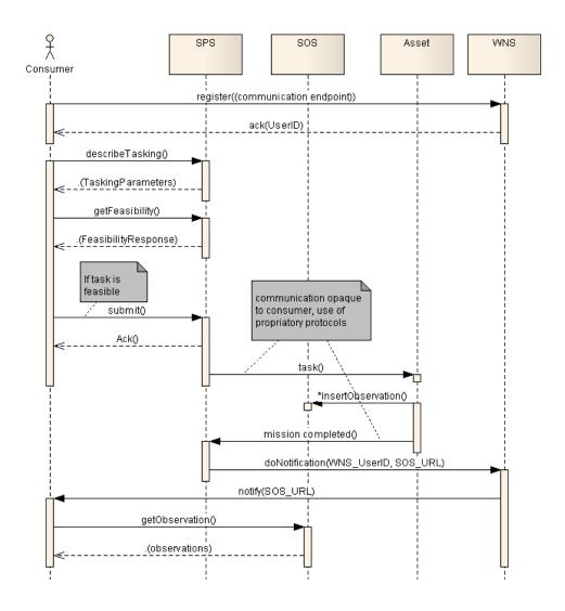
Figure 8-1: Typical sequence if data collection is requested
