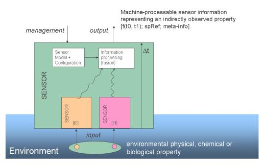
Figure 5-4: Model of a complex form of a Sensor
