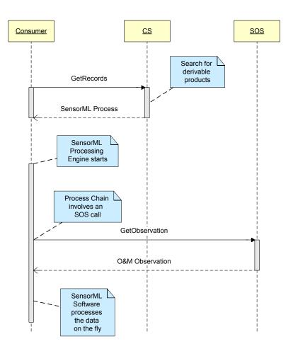
Processing SOS data using a SensorML Process Chain
