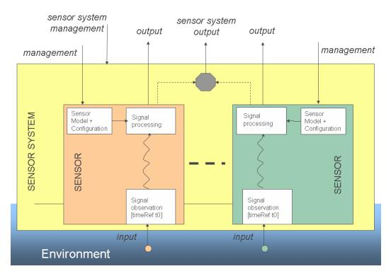
Figure 5-5: Model of a Sensor System
