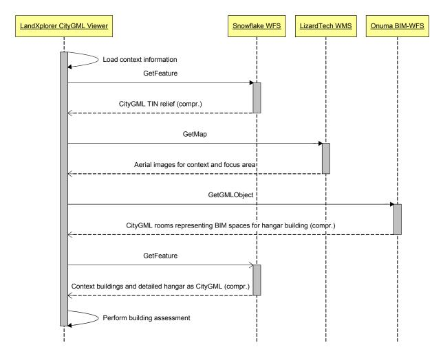
Figure B.1: Workflow sequence for LandXplorer CityGML Viewer.
