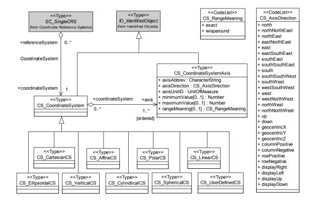
Figure 7 — CS CoordinateSystem package
